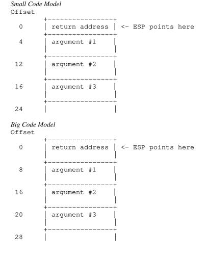
1. The return address is the top element on the stack. In a small code model, the return address is 1 double word (32 bits); in a big code model, the return address is 2 double words (64 bits).
