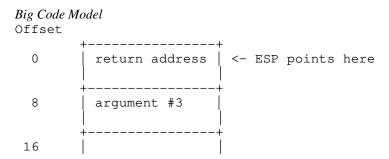
The return address is the top element on the stack. In a small code model, the return address is 1 double word (32 bits); in a big code model, the return address is 2 double words (64 bits).
