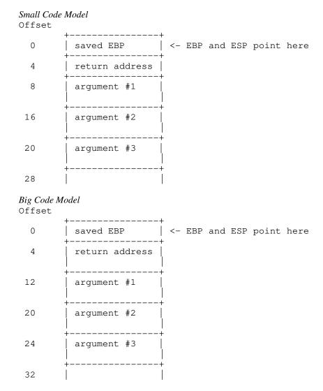
As the above diagrams show, the argument are all on the stack and are referenced by specifying an offset from register EBP.
