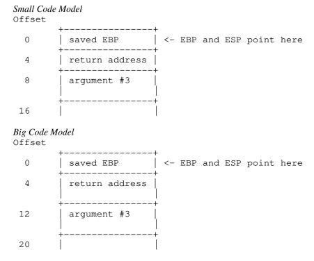
As the above diagrams show, the third argument is at offset 8 from register EBP in a small code model and offset 12 in a big code model.
