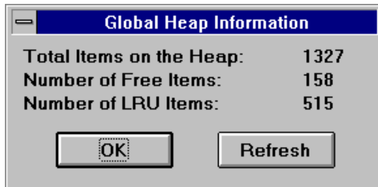
Figure 145. The Global Heap Information dialog provides a summary of global heap usage.
